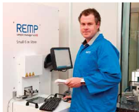
Automated Sample Storage: The REMP Small Sample Store is used to store all the samples required for an entire project, pre-aliquoted and ready for use. It has the advantage of being able to track each and every well of a 96 well plate using 2D barcoding and can deliver requested wells without removing the plate from the freezer.
