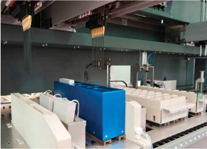
Automated Fusion Station: The robotic fusion platform can perform a hybridoma fusion from a single cell suspension. It is able to count both the spleen and myeloma cells and mix them in the appropriate ratios. It can also wash and centrifuge the cells and perform up to 8 fusions at a time.
