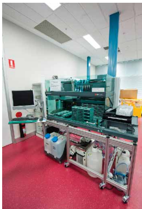
Automated ELISA station: The ELISA platforms at MATF are capable of performing an entire ELISA from plate coating right through to absorbance measurements. We use these robots for both the serum screen to ensure an animal has reached sufficient antibody titre as well as a conformation screen of the supernatant.
